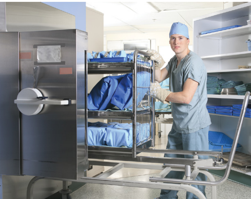
Hospital staff loading reusable devices into an autoclave for sterilization.
