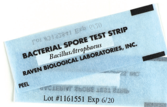
Biological indicators containing at least a million organisms of Bacillus atrophaeus are used to validate EO cycles.
