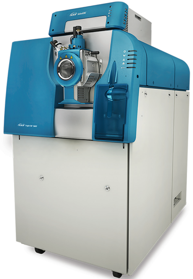
PBL's SCIEX TripleTOF 5600 mass spec system, generates high resolution MS and MS/MS spectra essential for extractable leachable studies.
